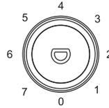
Set the temperature with the thermostat knob and select a position between 1 and 7. We recommend setting the appliance to position 3-4. The appliance will now cool continuously until the set temperature has been reached. Allow the appliance to reach the set temperature, before filling it with food. Usually this will take 2 to 3 hours. After that, you can set the thermostat to the required position and fill the appliance with food.
