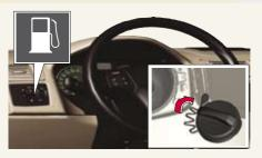
Press this button to unlock the fuel filler door. Hang the fuel filler cap on the hook while refueling.
