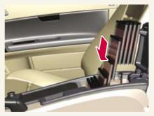
The deep center storage compartment has room for 10 CD jewel cases. These cases must be inserted with their spines upward in order to allow room for 10 CDs.
