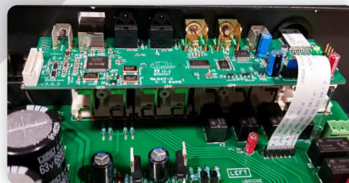
DA200 DAC board in the IN100 Signature
