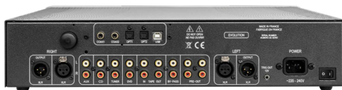
PR300 Evolution with DA200 DAC board rear view.
