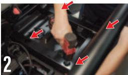
REMOVE 4 BOLTS IN SEAT MOUNT AS SHOWN
