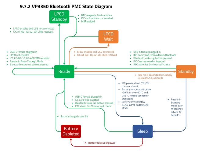
Note that pressing the reader's reset button will force the reader into a power off/battery depleted state and then restart the reader in the Ready state.
