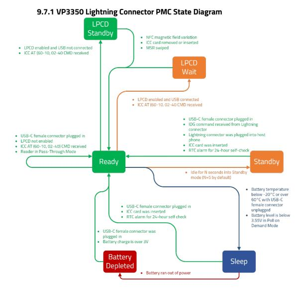
Note that pressing the reader's reset button will force the reader into a power off/battery depleted state and then restart the reader in the Ready state.
