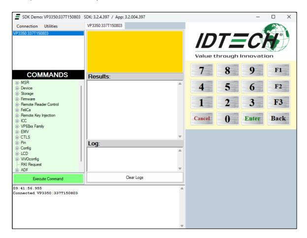
The Universal SDK Demo app displays VP3350's available commands in a command tree, as shown above. Single-click on a command to populate the lower-right panel of the window with optional settings relevant to the command (for example, "Amount" and "Start EMV Additional Tags" above). In some cases, text fields appear, allowing users to enter custom values.
