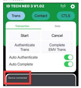
3. Select the **Start** button. The message pane displays **Start Transaction info ERROR: ID- "RETURN\_CODE(rawValue:61024)", message: Data not exist**. This error indicates the device has not yet been configured.
