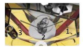
5: Fit the pump cover in place and gently tighten the screw.
