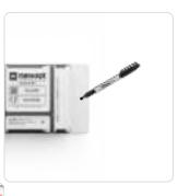
Hold the device against the asset and use the mounting holes of the device as a stencil to mark the drill positions. Drill with a 6.5 mm to 7.0 mm drill bit (Gauge Size: G/H/I). WARNING. DO NOT use the Globehopper as a drill guide, as this will damage the enclosure.
