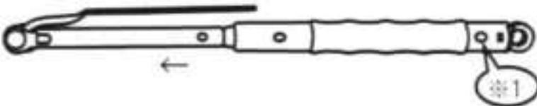
**STEP4.** Hold the handle of B and pull up A for the longest length.
