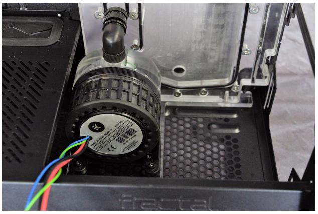
**Step 10**: Secure the Panel/D5 Mounting Plate with the provided 2x fan screws in the fan screws specified in the image below.
