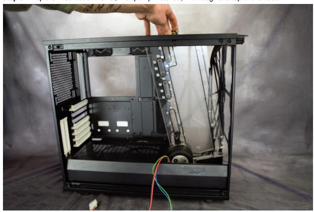
**Step 9**: Orient the Panel and pump as pictured below. Once it is in the correct position, flip the case on its back side so you have access to the bottom of the case.
