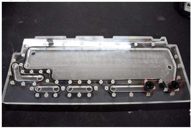
**Step 5**: Slide the Bitspower Dual G1/4" Adjustable Aqua Link Pipe fittings together to install the pump on the distribution panel.
