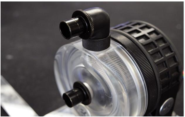
**Step 4**: Install the other halves of the 2x Bitspower Dual G1/4" Adjustable Aqua Link Pipe's in the specified ports on the Distribution Panel.
