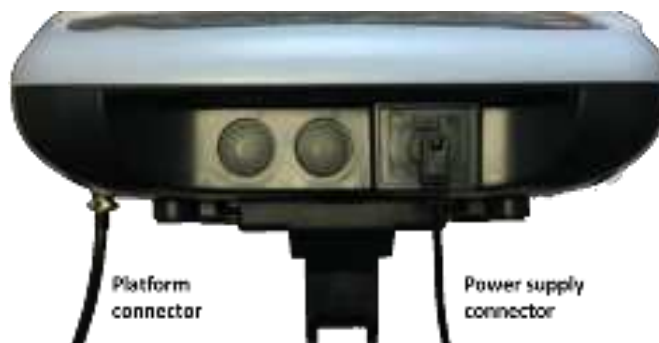
Fig. 5 Signal cable plugged into back of the indicator
