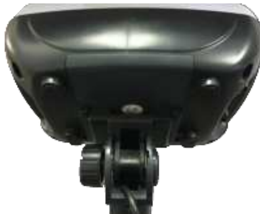
Fig. 4 Slide indicator head onto column bracket
