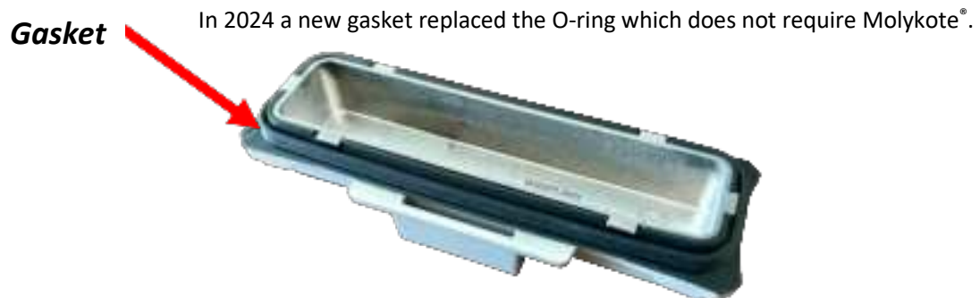
Figure 43: New End Cap Gasket
