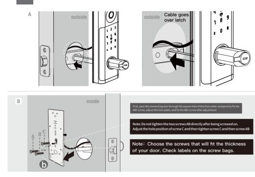
Install front panel and interior mounting plate
