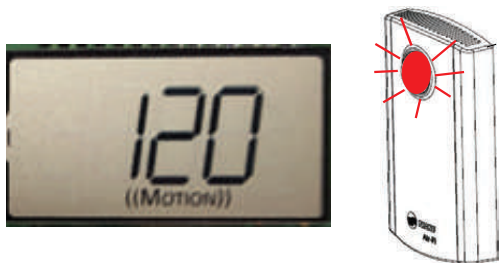
Figure 37. Sensor eye turns red when motion is detected
