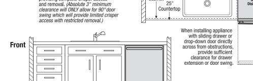
appliance with sliding drawer or drop-down door adjacent to wall, cabinet, or other obstruction that extends beyond front edge of appliance, allow 2" minimum clearance between drawer or door and obstruction.
