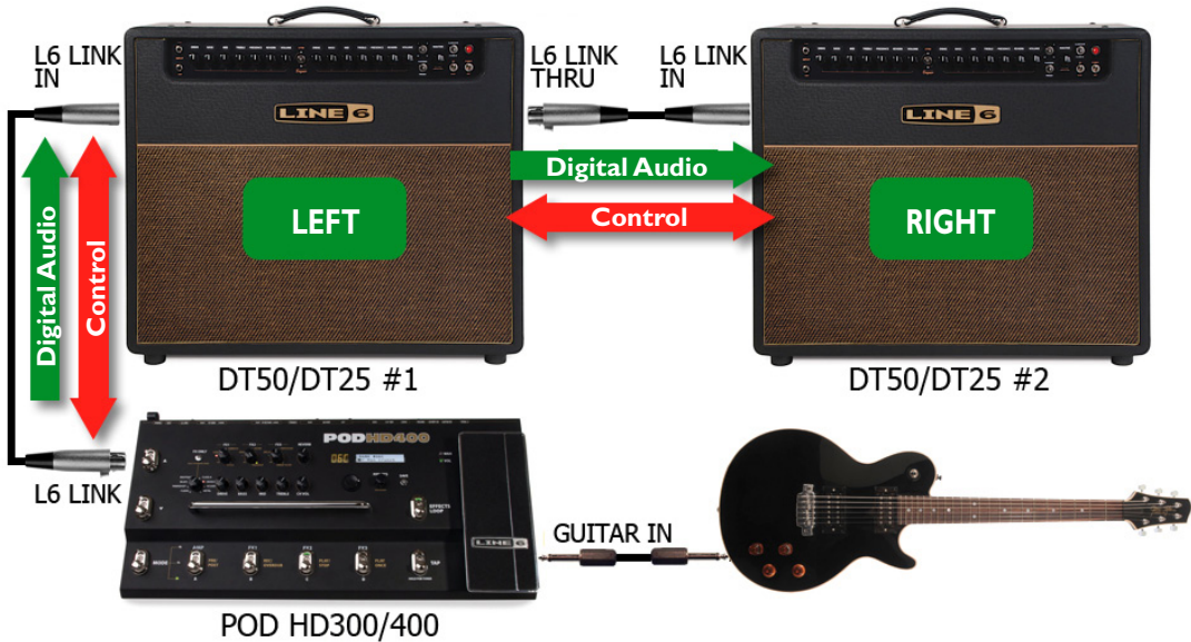
POD HD with a stereo, dual DT Series amplifier setup, using L6 LINK
