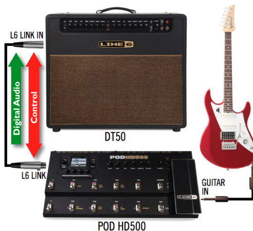
POD HD500 connected to DT50 using L6 LINK
