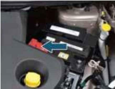
Motor Compartment Fuse Box
