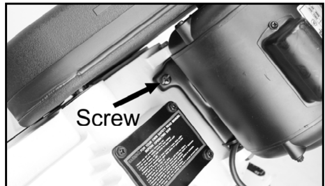
Figure-14 Loosening the tension on the belt
