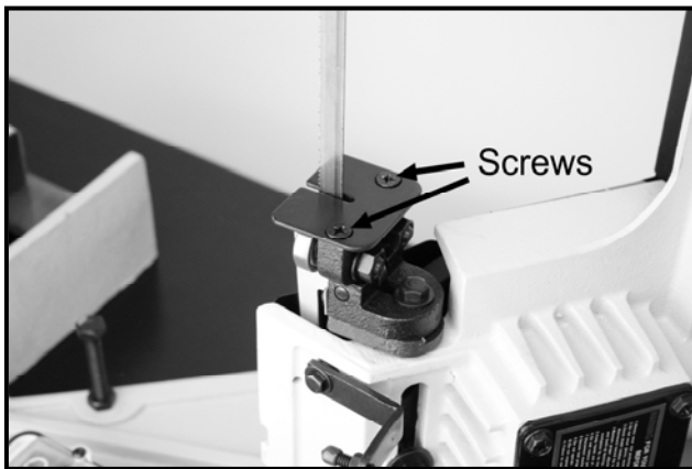
Figure-11 Removing the two screws
