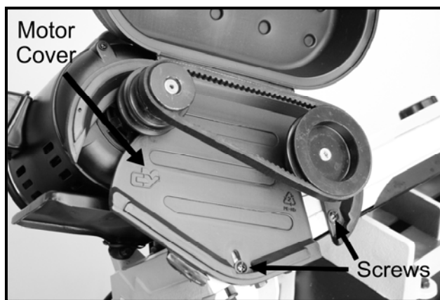
Figure-9 Installing the motor cover
