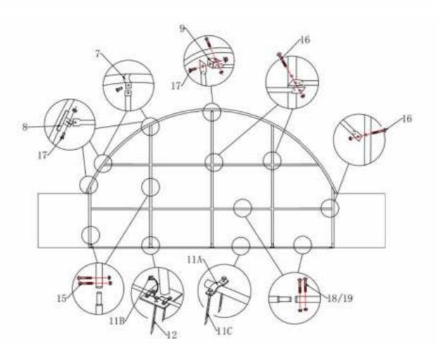
According to above Figure to find out all spare parts for back wall, connect them together by use screw, make sure the spacing. There are Expansion screw for base plates.
