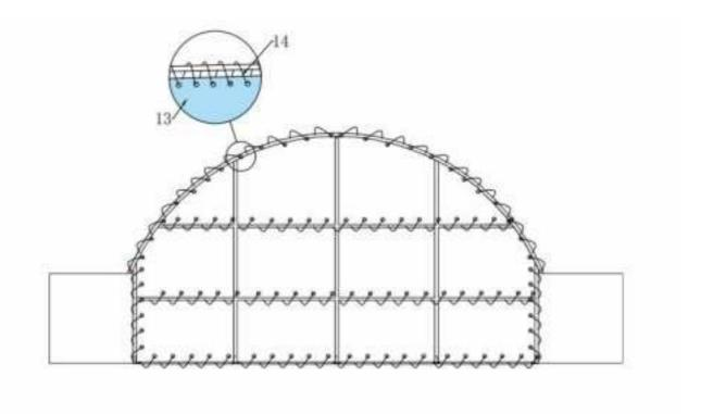
Find out the back cover(No.13), use ropes(No.14) to tie it to the back wall. Adjust and tighten them once per month after assembly to make sure them works perfect.
