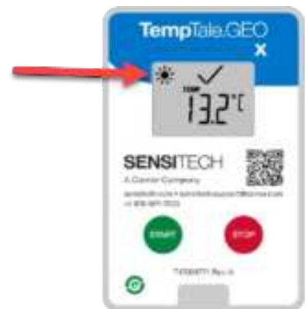
Monitor turned on when sun icon blinks.
