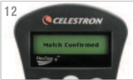
Repeat the process for the third alignment star. When the telescope has been aligned to the final star, the display will read "Match Confirmed." Press UNDO to display the names of the three bright objects you aligned to, or press ENTER to accept these three objects for alignment.
