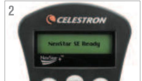
2 The display reads "NexStar SE Ready." Press ENTER to begin the alignment procedure.
