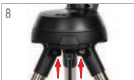
Tighten the captive mounting bolts under the tripod head to secure the mount. Once tightened, confirm that the bolts are fully seated and that the mount is firmly attached to the tripod.
