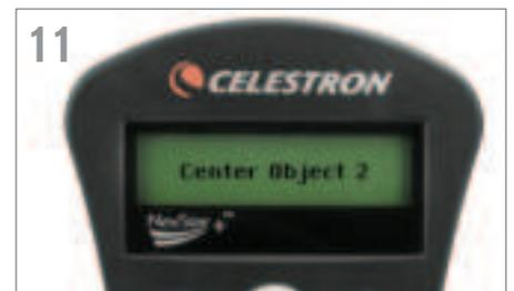
11 For the second alignment object, choose a bright star or planet that's as far from the first one as possible. Use the directional arrow buttons to center it in the finderscope and press ENTER. The motors will slow. Center it in the eyepiece and press ALIGN.
