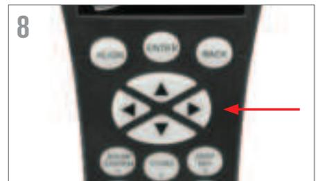
8 The mount is now ready for alignment. From this point on, do not move the telescope by hand—use only the directional slew buttons on the hand control.
