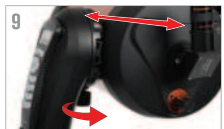
To adjust the balance or remove the tube from the base, loosen the quick-release clamp knob and slide the tube back towards the rear cell of the tube. Hold the tube firmly when mounting or dismounting. Ensure the dovetail clamp is tight before releasing the tube.
