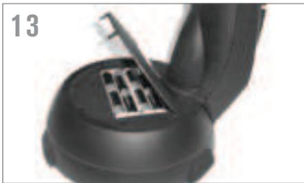
Remove the battery cover from the center of the base by gently lifting on the round portion of the cover. Insert 8 AA batteries into the holder and reattach the battery cover. Be careful to insert the batteries in the correct polarity.
