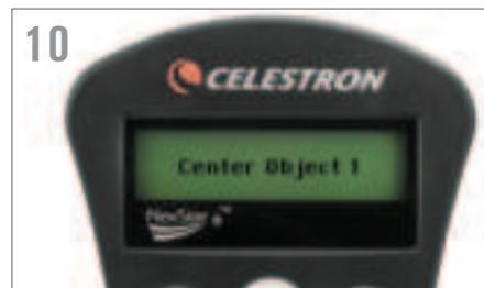
10 The hand control will now prompt you to center the bright object in the eyepiece. The motors will automatically slow down to help with fine adjustments. Once the object is centered, press ALIGN to accept it as your first alignment point.
