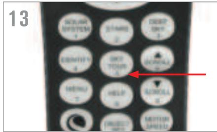
Now that your telescope is properly aligned, you are ready to find your first object. Press the SKY TOUR button (number 5 on the keypad) on the hand control. The hand control will display a list of objects that are visible, above your horizon, for the date and location you entered.
