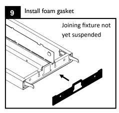
Insert the foam gasket onto the fixture end. Slide the gasket over joiner pair and ensure the gasket is firmly seated inside the housing.
