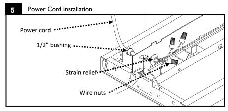
Insert supplied 1/2" bushing into 1/2" electrical knockout on access panel. Route supplied power cord through bushing. Crimp supplied strain relief onto power cord insulation (recommend Heyco Tool PN0019(R12). Ensure power cord does not have excess slack or is too tight. Complete necessary electrical connections (by others) in compliance with local codes.
