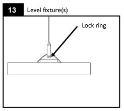
Loosen cable gripper lock ring, adjust sling mount(s) to level fixtures. Tighten lock ring when complete at all mount locations. Cut excess suspension cable if necessary.
