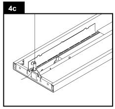
Open the electrical panel to access the wiring cavity.
