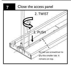
Ensure the electrical connectors are tucked inside the wire cavity. Push down on the lid while simultaneously twisting the flat blade screwdriver, the panel tab will lock into place. Repeat at the other screwdriver slot location. For standalone fixtures skip ahead to step 12.
