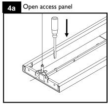
Identify power feed location on fixture. Insert a medium size flat blade screwdriver into slots on access panel.
