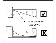
Re-install the upper diffuser (SHINY SIDE facing DOWN). If applicable, install optional 75 or 100% downlight reflectors on top of upper diffuser in correct orientation.
