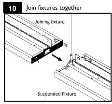
With two people, insert the joining fixture into the suspended fixture. The joiner pair will engage into the suspended fixture crossplate. Support the other end of the joining fixture with a suspension cable as in steps 2-3.
