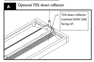
FloatPlane Fixtures available with a factory installed, perforated 75% down reflector. For best optical performance, reflector must be installed as shown, SHINY SIDE facing UP. Note the 75% down reflector is installed on top of clear acrylic upper diffuser.
