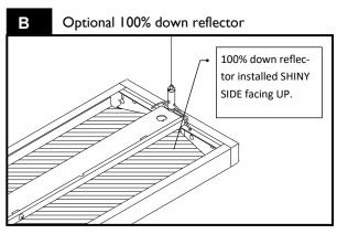
FloatPlane Fixtures available with a factory installed, solid 100% down reflector (shown as hatched lines). For best optical performance, reflector must be installed SHINY SIDE facing UP. Note the 100% down reflector is installed on top of clear acrylic upper diffuser.
