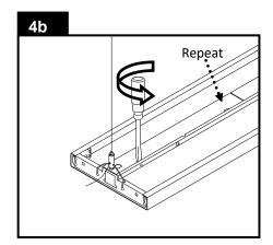
Twist the screwdriver and the tab on the access panel will POP UP. Repeat steps 4 at the other tab on the access panel.
