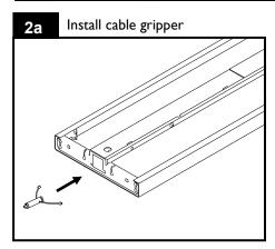
Insert sling cable gripper into crossplate holes as shown.
