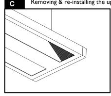
If the fixture is mis-handled during installation, a shadow may appear in the luminous window. This is caused by the upper diffuser being pushed below the LED.
