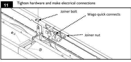
Ensure both fixtures are horizontal and suspended at the same height. Snug jointing nuts using 3/8" nut driver, align the fixture housings for best aesthetic before final tightening. Complete necessary electrical connections in compliance with local codes. Close all wire access panels (step 7) when complete.
