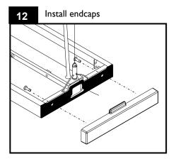
Insert the foam gasket onto the fixture end and ensure the gasket is firmly seated inside the housing. Using supplied Phillip screws, snug the endcap in place. Align the endcap to fixture housing before final tightening. Cut excess suspension cable if necessary.
