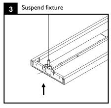
With 2 people, raise the fixture up to the suspension cables and feed through grippers. Set fixture to desired height.
