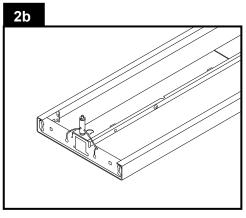
Pivot the cable gripper up. Repeat at other end of light fixture.
