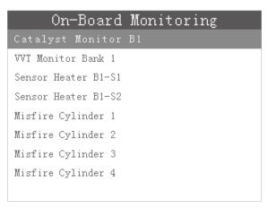
3. Use the UP / DOWN / LEFT / RIGHT key to highlight a test group and press the OK key to confirm, A screen with details of the selected sensor displays. Use the UP/DOWN arrow
