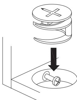
head should be in the centre of the cam lock when the two panels are joined.
