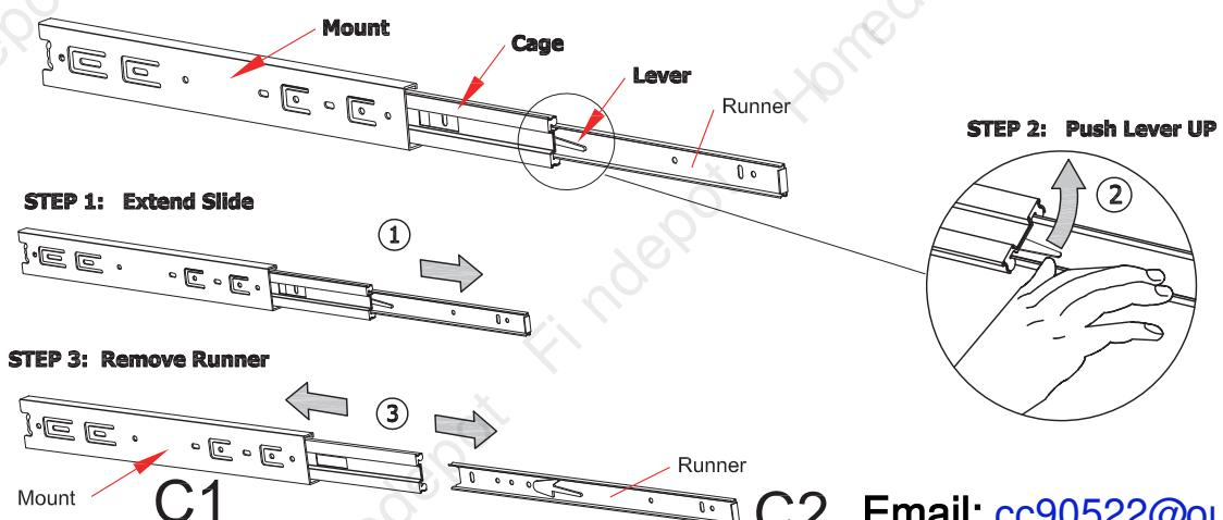
The guide rail needs to be divided into two parts: C1 and C2.
