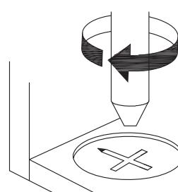
Turn cam lock clockwise to tighten.
