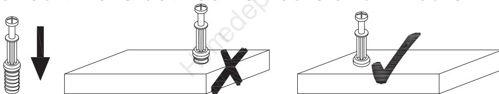
Tighten quickfit until shoulder is flush with panel. Do not overtighten or undertighten.
