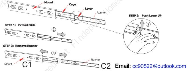
The guide rail needs to be divided into two parts: C1 and C2.
