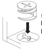
head should be in the centre of the cam lock when the two panels are joined.
