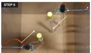
6. **UV Lamps and Ballast Position:** The lamps should be positioned towards a central point in the middle of the unit's aluminum reflection chamber.
