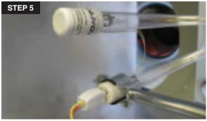
5. Insert the white-plug into the UV Lamp's 4 pins. The plug will only fit in two of four ways. Either way is fine. The exposed wire-set is Teflon coated and is resistant to UV exposure.
