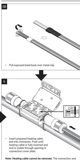
end seal are designed to be installed only once; the heating
