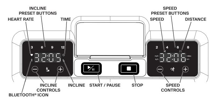
**INCLINE:** Shows the current Incline setting of the deck.
