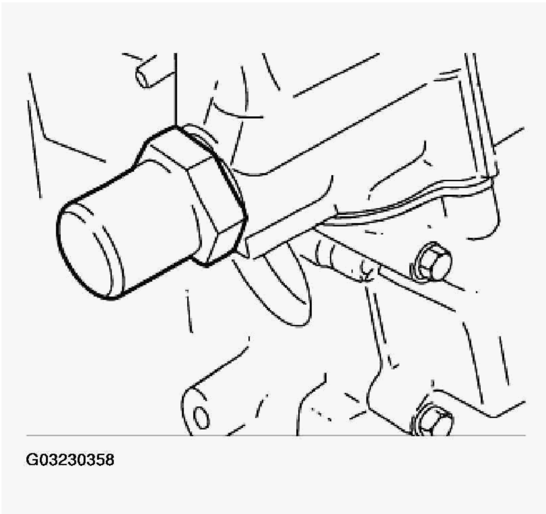
Fig. 316: Locating Cylinder For Tensioning Piston Courtesy of BMW OF NORTH AMERICA, INC.
