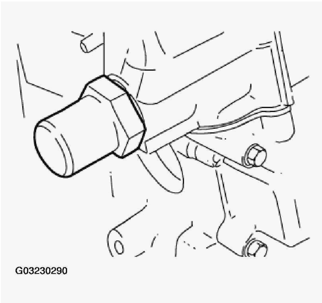
Fig. 248: Removing Cylinder For Chain Tensioning Piston Courtesy of BMW OF NORTH AMERICA, INC.
