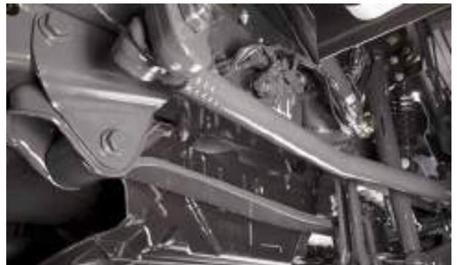
Front spring, 3.6 t, parabolic (Q1J)
