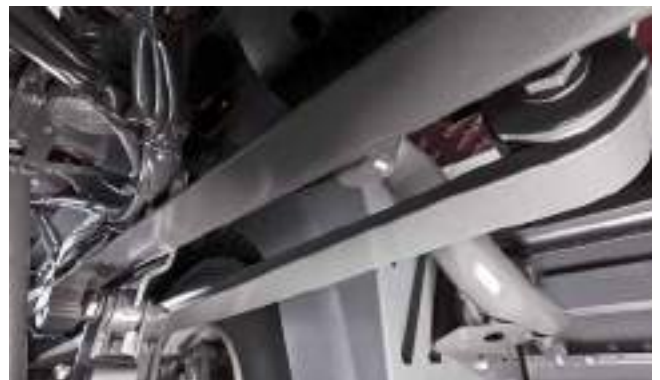
Rear spring, 5.0 t, parabolic, 1-leaf (Q2N)
