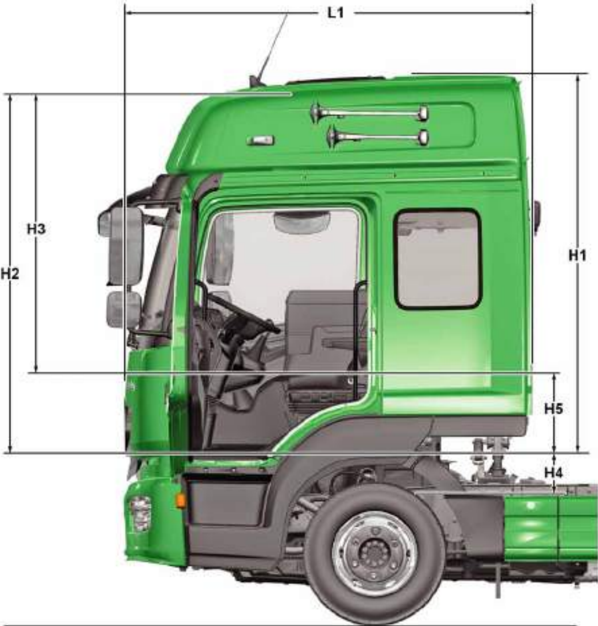
Cab dimensions based on the example of platform vehicle with L-cab, engine tunnel 460 mm, ASH 140
