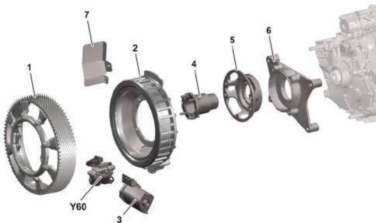
Permanent magnet retarder (B3G) on transmission G 90-6
