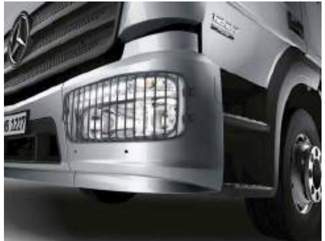
Stone impact protection, metal, for headlamps (L4Z)
