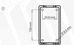
Attach mounting plate to the surface. Please leave required space from all sides for cables and loudspeaker angle adjustment.
