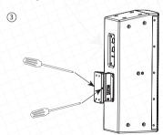
Place loudspeaker with attached bracket onto mounting plate. Fix the two security screws on both sides of the bracket to prevent loudspeaker removal from the plate.
