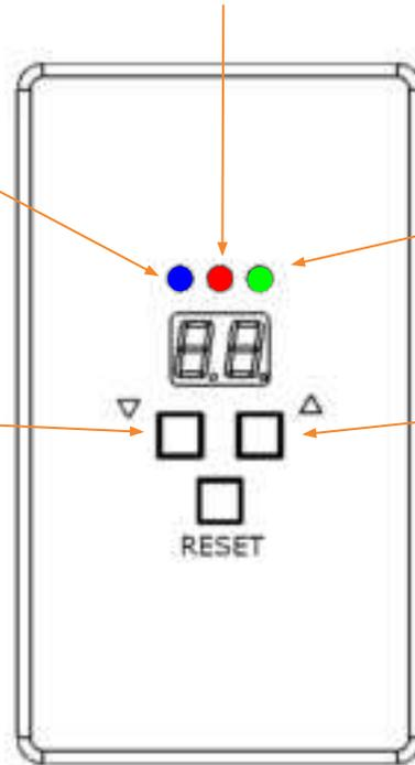
If you experience any issues at this step, connect to the robot in the tablet and manually change the channel to any other number. You may then change the channel on this box to match that newly set channel.
