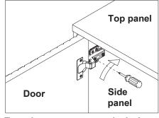
Turn the screw counterclockwise a little as shown to make the gap bigger
