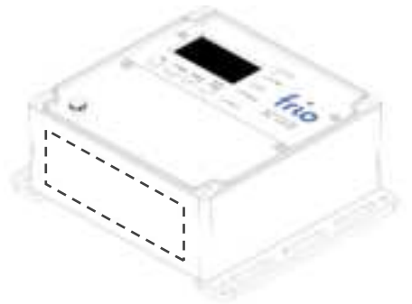
Figure 1: Frio S1 controller showing the bottom side where to drill wiring holes.
