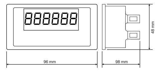
**Weight:** 170 g; **Enclosure:** Self-extinguishing PC/ABS material, black.
