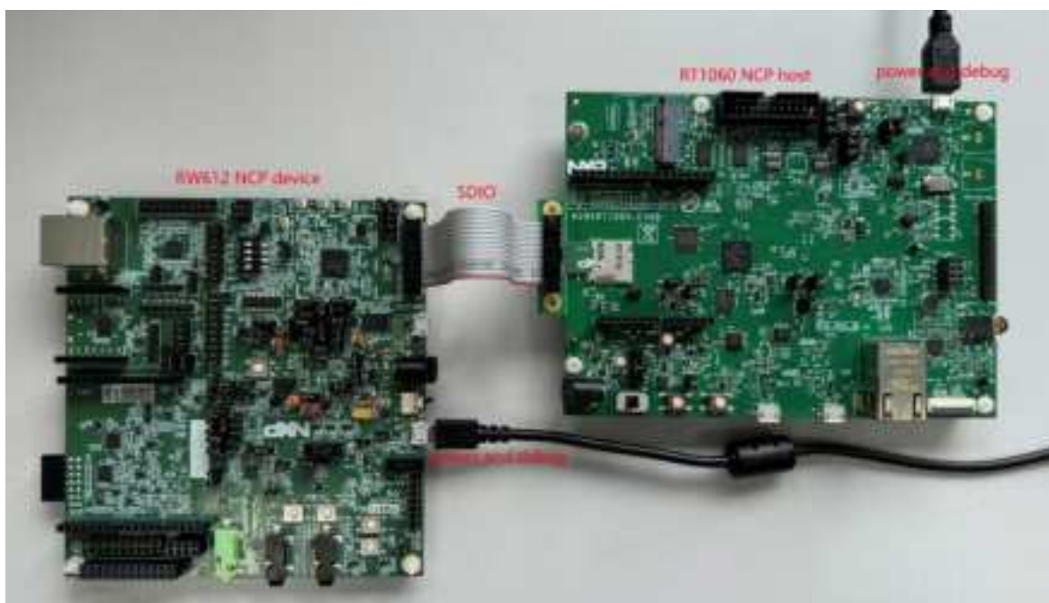
Figure 7. Connection between i.MX RT1060 board and RW612 board with the mini-SDIO cable
