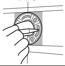
Step 02 Drill Hole on Tile. Hold the drill TIGHT in position and press gently on tile surface to create a groove then slowly extend the groove to a hole.
