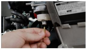
**31.** Install the new jet into the carburetor. As mentioned earlier, make sure you're installing the correct jet for your model of generator and for the altitude. After you install the new jet, don't throw away the old one.
