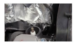
**16.** Finally remove the housing to gain access to the carburetor. Pull the spark plug wire off the spark plug.
