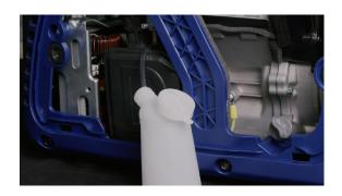
**8.** Locate the clear plastic hose from the float that is exiting out the bottom of the generator, and place a gasoline safe container under it to catch the drained fuel.
