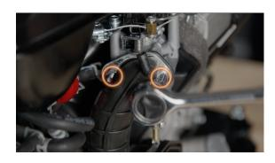
**27.** Remove the 2 nuts that secure the air cleaner to the carburetor.
