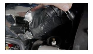
19. Pull the spark plug wire off the spark plug.
