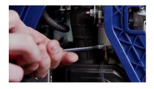
**9.** Loosen the float bowl drain screw until fuel is seen draining from the float bowl. Allow any fuel to drain, then tighten the float bowl drain screw.
