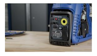
**14.** Pull the front panel off, leaving the wires behind the control panel attached.
