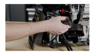
**28.** Remove the air cleaner assembly. Be sure the paper gasket between the air filter and carburetor is not damaged.
