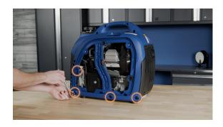
**10.** Continue with the removal of the generator cover. Remove the 3 bolts at the bottom of the engine access panel and the single bolt near the front air vents.
