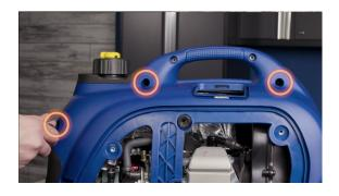
**10.** Remove the 3 screws at the top of the housing.
