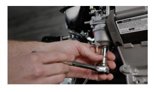
**29.** Remove the bolt from the bottom of the carburetor float bowl. There may be some leftover fuel in the carburetor so have a rag handy to clean any spills.
