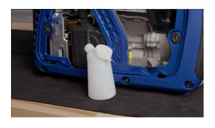
7. Locate the clear plastic hose from the float that is exiting out the bottom of the generator, and place a gasoline safe container under it to catch the drained fuel.
