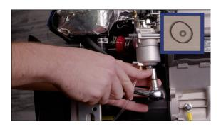
**25.** If they are damaged, replace the o-ring where the bowl meets the carburetor, and the bolt seal on the bottom of the carburetor, with the parts supplied in the kit. Re-bolt the bowl onto the bottom of the carburetor.
