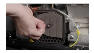
**18.** Remove the screw in middle of the air cleaner and remove the foam filter.
