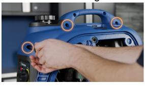
11. Remove the 3 screws at the top of the housing.
