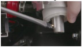
**24.** Remove the old jet, and install the new jet into the carburetor. As mentioned earlier, make sure you're installing the proper jet for your model of generator and for the altitude. After you install the new jet, don't throw away the old one.
