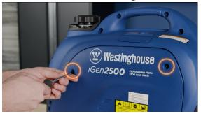
**6.** Remove the 2 screws that secure the engine maintenance panel to the frame. Keep track of the screws and bolts as you disassemble the generator housing.
