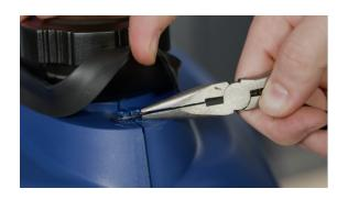
**15.** Using a pair of needle nose pliers, remove the clip located under the rubber fuel collector.
