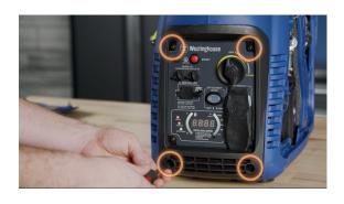
**12.** Remove the 2 screws at the top of the control panel and the 2 screws \*under\* the control panel.
