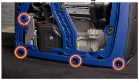
**9.** Continue with the removal of the generator cover. Remove the 3 bolts at the bottom of the engine access panel and the single bolt near the front air vents.
