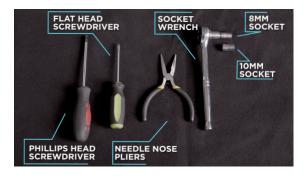
2. To perform this installation, you'll need a Phillips head screwdriver, a flat head screwdriver, a pair of needle nose pliers, a socket wrench, an 8mm socket, and a 10mm socket.
