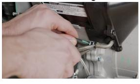
**21.** Unclip and pull off the breather tube connected to muffler.
