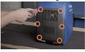
**14.** Remove the 6 screws that hold the muffler to the generator and remove the muffler.
