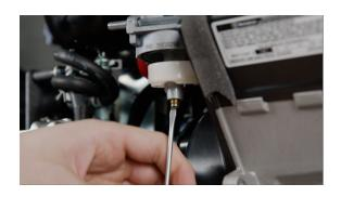
**30.** Use the small flathead screwdriver to carefully remove the jet. Make sure the main nozzle stays in the carburetor. If it falls out, replace it in the correct orientation.
