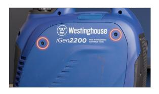
**5.** Remove the 2 screws that secure the engine maintenance panel to the frame. Keep track of the screws and bolts as you disassemble the generator housing.
