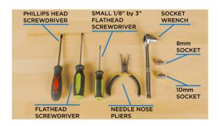
3. To perform this installation, you'll need a Phillips head screwdriver, a standard sized flathead screwdriver, a small 1/8in by 3in flat head screwdriver, a pair of needle nose pliers, a socket wrench, an 8mm socket, and a 10mm socket.
