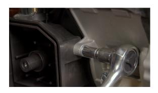
**20.** Remove the bolt on the right side that secures it to the engine mount.
