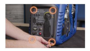
**11.** Remove the 2 screws at the top of the control panel and the 2 screws \*under\* the control panel.
