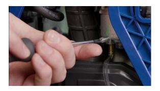
**8.** Loosen the float bowl drain screw until fuel is seen draining from the float bowl. Allow any fuel to drain, then tighten the float bowl drain screw.
