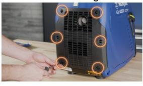
**16.** Remove the 6 screws that hold the muffler to the generator and remove the muffler.
