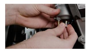
**32.** If they are damaged, replace the o-ring where the bowl meets the carburetor, and the bolt seal on the bottom of the carburetor, with the parts supplied in the kit. Re-bolt the bowl onto the bottom of the carburetor.
