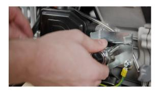
**23.** Remove bolt holding the carbon canister bracket and pull the bracket off.
