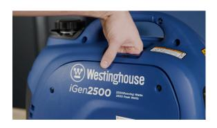
7. Slide off the spark plug access cover, and push on the maintenance panel to remove it.
