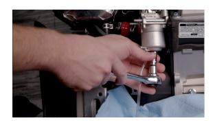
**23.** Remove the bolt from the bottom of the carburetor float bowl. There may be some leftover fuel in the carburetor so have a rag handy to clean any spills.
