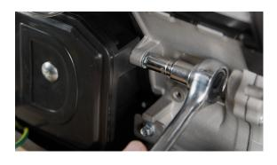
**24.** Remove the bolt on the right side of the air cleaner box that secures it to the engine mount.
