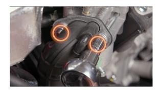
**21.** Remove the 2 nuts that secure the air cleaner to the carburetor.
