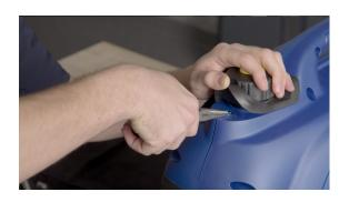
**13.** Pull the front panel off, leaving the wires behind the control panel attached. Using a pair of needle nose pliers, remove the clip located under the rubber fuel collector.
