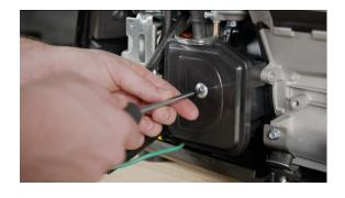
**25.** Remove the screw in middle of the air cleaner and remove the foam filter.
