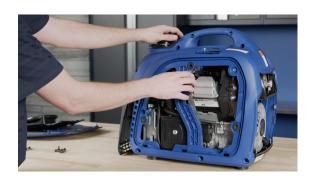
**18.** Finally remove the housing to gain access to the carburetor.
