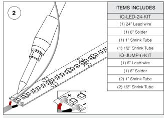
Solder lead wire onto solder pad. Confirm postive (+) and negative (-) are matched up correctly before soldering. BLACK wire is typically negative, RED wire is typically postive.
