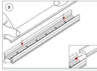
Flat Lenses: Apply uniform pressure until the extrusion and lens snap securely together.
