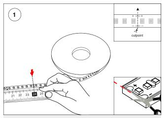
Measure and cut LED strip to desired length with scissors along the cut point.
