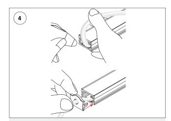
Add glue inside the end cap and glue around edges to secure end cap in place. Do not allow glue to come in contact with LED.
