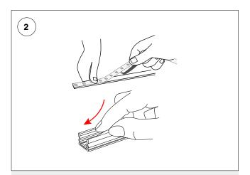
Peel back 0.5" of the VHB tape's protective film on one end of LED and use firm pressure to adhere it to the desired surface, avoiding air bubbles. Continue peeling the film and adhering the strip in small sections until the entire length is installed.
