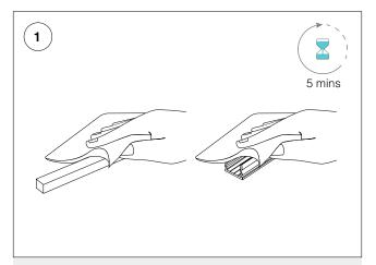
Using a 50/50 alcohol mix throughly clean, the surface of the extrusion and the multi-tray surface. Allow time to dry (about 5 minutes).
