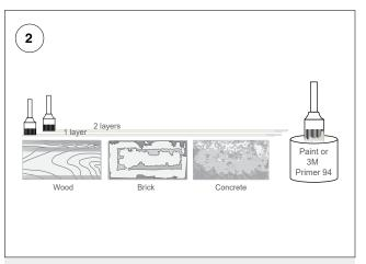
For porous materials (Wood, Brick, Concrete etc.) apply two layers of paint or primer to the surface. This will help create a better bonding surface for these materials. These can be purchased from a local hardware store.
