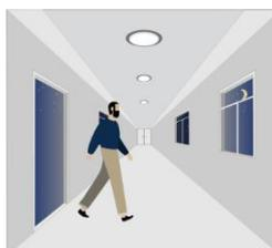
When motion is detected and the ambient brightness is too low, the light will be turned on to 100%.
