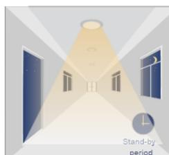
The light will be dimmed to standby value, after the hold time. When the standby-time is setted to 0 sec., sensor switch off the light after the hold time.
