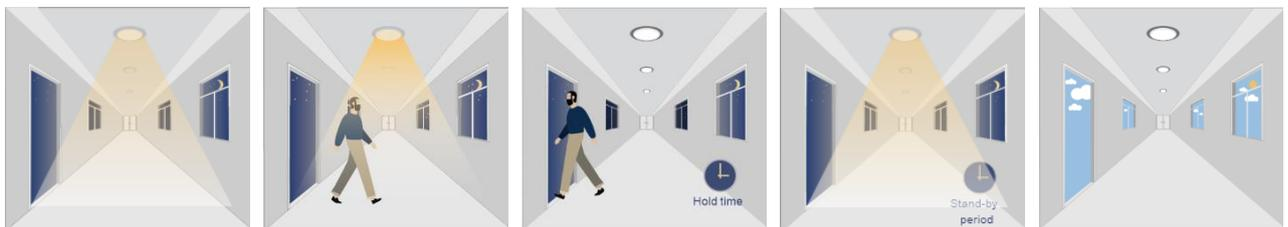
When insufficient ambient brightness is detected, sensor turns on light to standby dimming value, even if motion is not detected.
