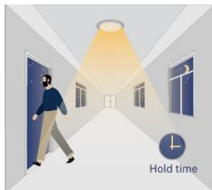
When no motion will be detected, the light keep on 100% brightness for the setted hold time.
