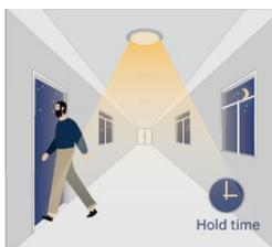
When no motion is detected, the light keep on 100% for the hold time.
