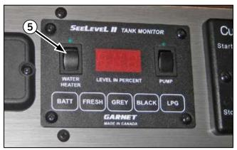
The water heater is equipped with a preset water temperature control. The burner will bring the water temperature up to the desired level and then automatically shut off. The burner automatically reignites when necessary to maintain the preset water temperature.
