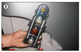
**Exterior Flood Light (1)** - Unclip the top cover (2) and replace the bulb. Reinstall the cover.
