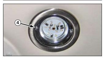
**Interior Shower Light (5)** - Unclip the cover (6) and replace the bulb. Reinstall the cover.
