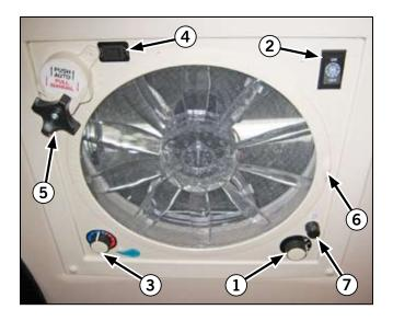
NOTE: at 1/3 open, fan blade exhaust efficiency is reduced to 90%. After adjusting, always push the knob (5) up to ensure it is locked into the "AUTO" position.
