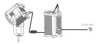
Note: Do not plug or unplug the power cord or connecting cable when the power is turned on, otherwise injuries may occur.
