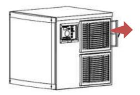
A Note: Be careful when doing the condenser cleaning as the edges of the fins are sharp.
