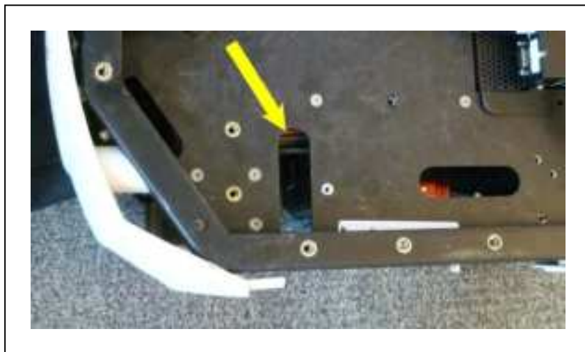
Figure 9-8. Cutout in Payload Bay for Cables
