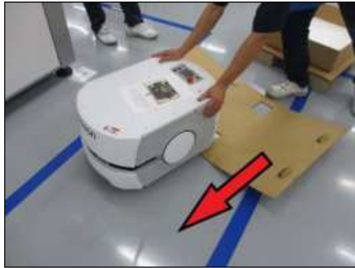
Figure 3-10. Robot Rolled onto the Floor
