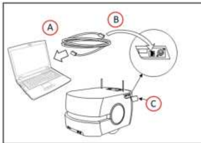
Figure 4-1. (A) PC, (B) Cat 5 Ethernet, and (C) Maintenance Access Panel
