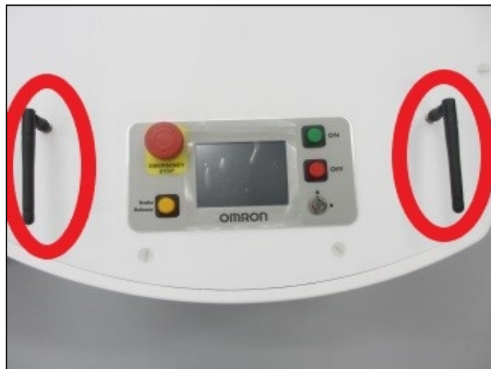
Figure 3-11. Robot Antennas Circled in Red
