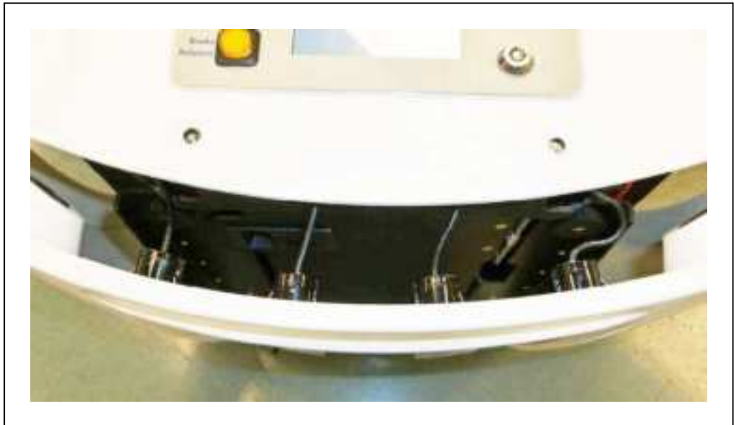
Figure 8-20. Sonar Leads, with Connectors Still in Chassis
