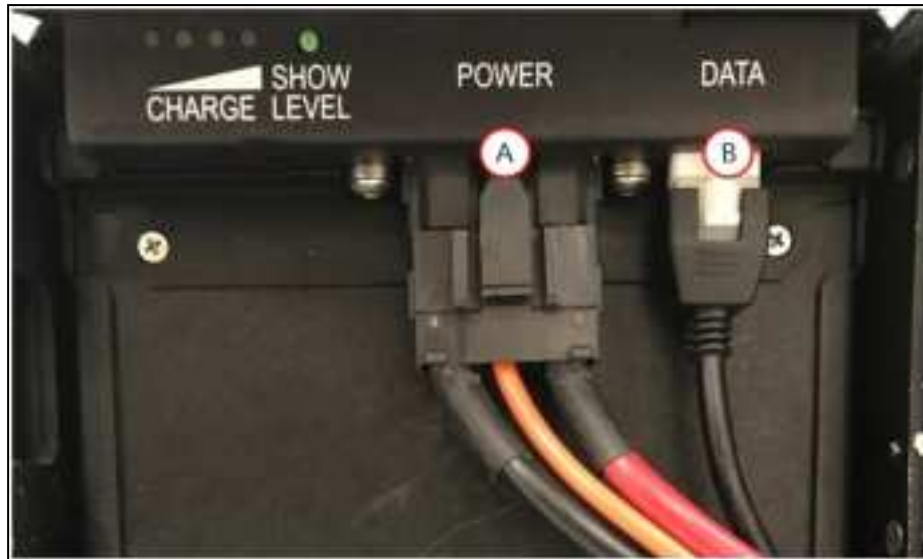
Figure 8-6. Battery Cable Connectors, (A) Power and (B) Data
