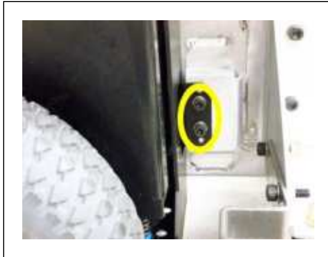
Figure 8-16. Mounting Screws at Bottom-Right of Drive Assembly
