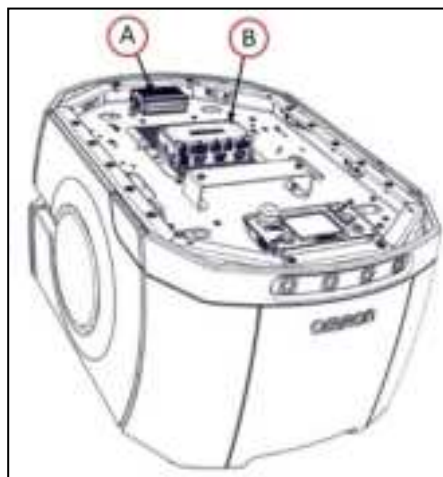
Figure 8-11. (A) Sonar Controller, (B) Core
