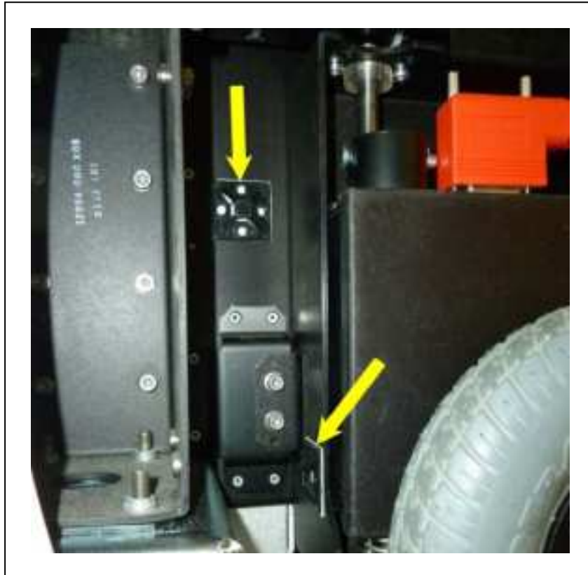
Figure 9-3. Cable-tie Anchors Behind Right Wheel
