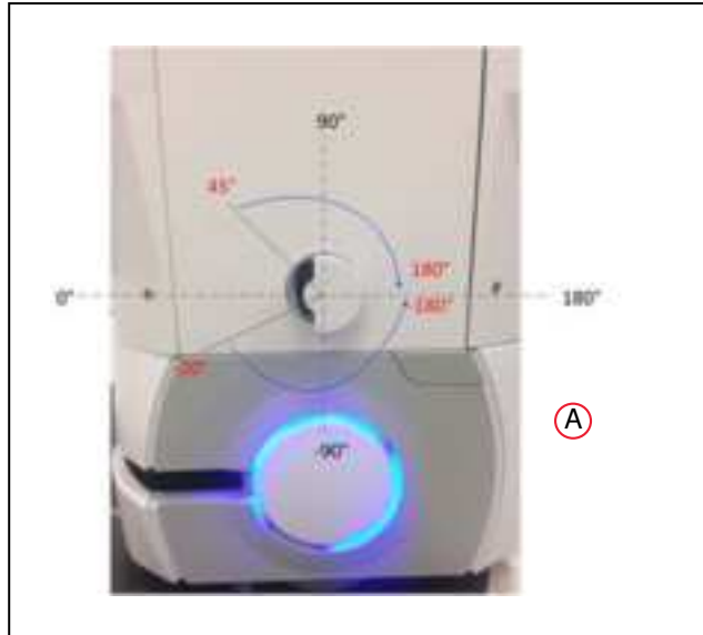
Figure 9-44. Left Side Laser (Laser 4), (A) This Laser is Flipped Upside-Down
