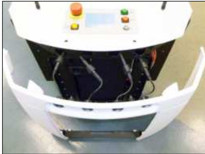
Figure 8-10. Sonar Connectors with Connectors Exposed
