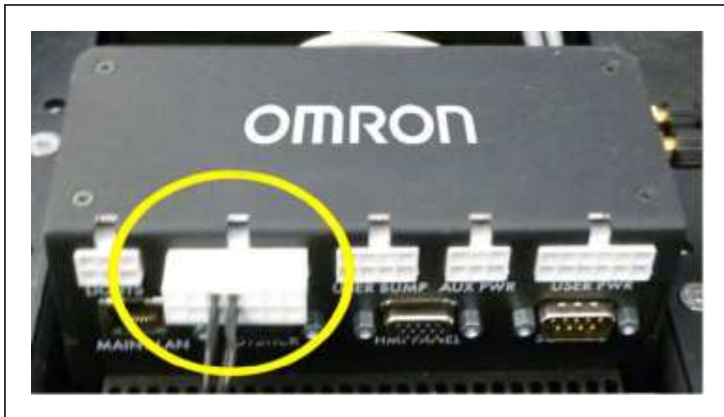
Figure 9-9. Upper Rear of Core, Showing AUX PWR Port
