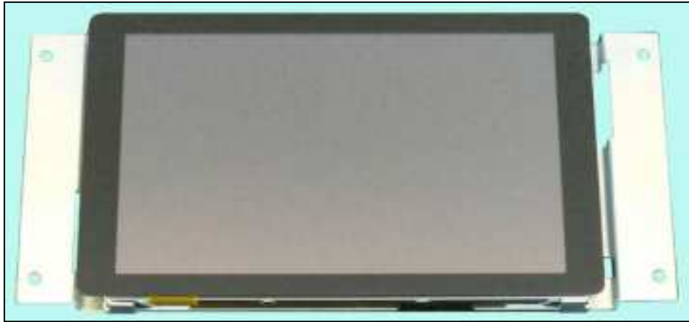
Figure 9-49. Front of touchscreen with Bracket
