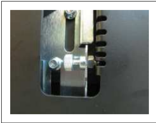
Figure 3-24. Docking Station Contact Adjusting Pull-Knob
