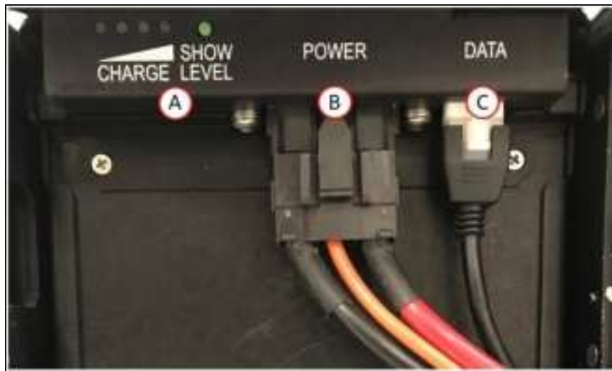
Figure 7-2. (A) Battery LEDs and Push-Button (Show Level), (B) Power Cable, and (C) Data Cable
