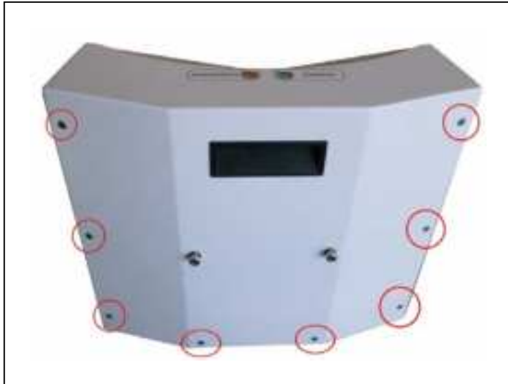
Figure 8-9. Docking Station Rear Cover Screws (8 of 10)
