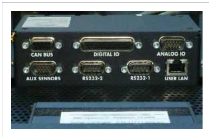
Figure 9-10. Upper Front of Core, Showing RS232 Ports
