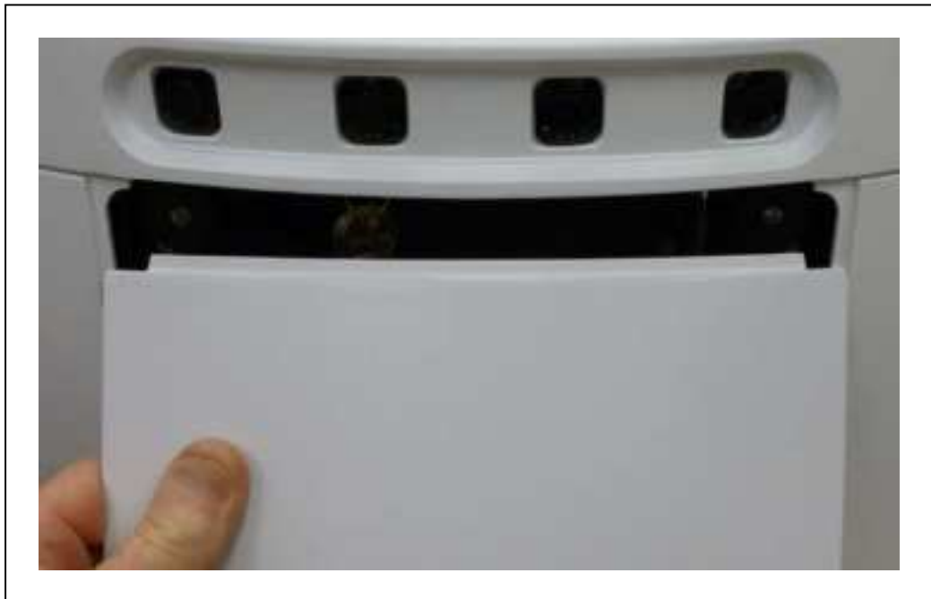
Figure 3-14. Lowering the Battery Door Platform Skin
