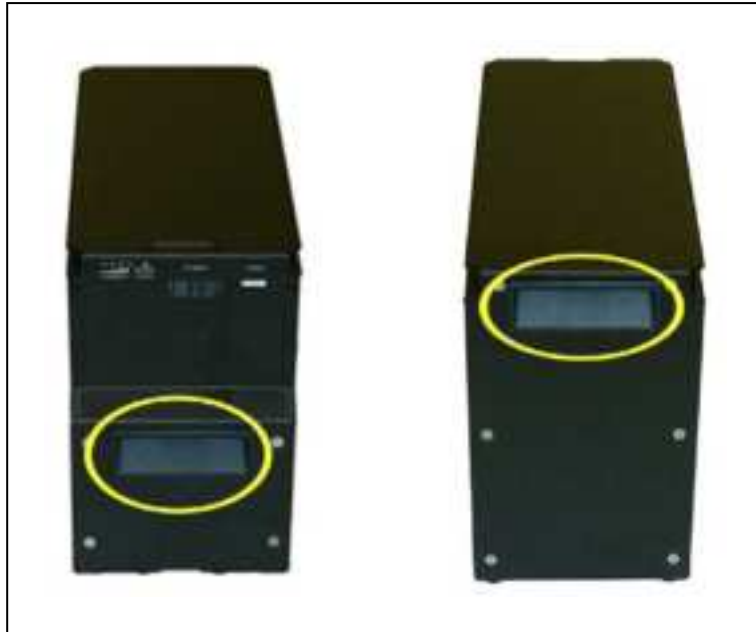
Figure 8-4. Battery Recesses, for Gripping
