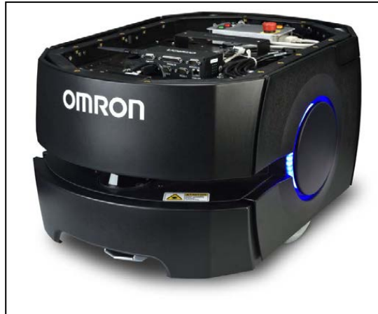
Figure 1-7. LD Platform OEM with ESD Skins
