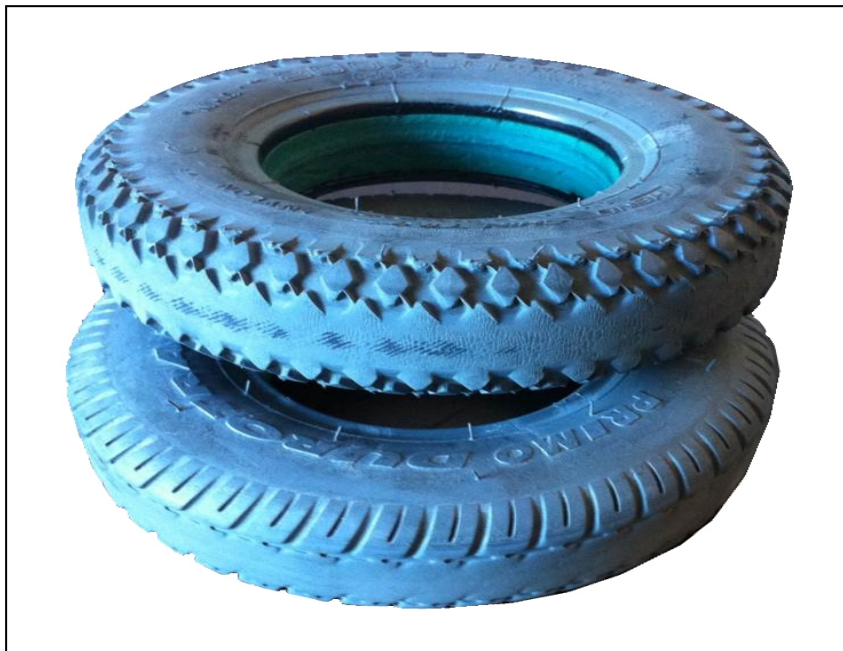
Figure 8-12. Samples of Tire Wear
