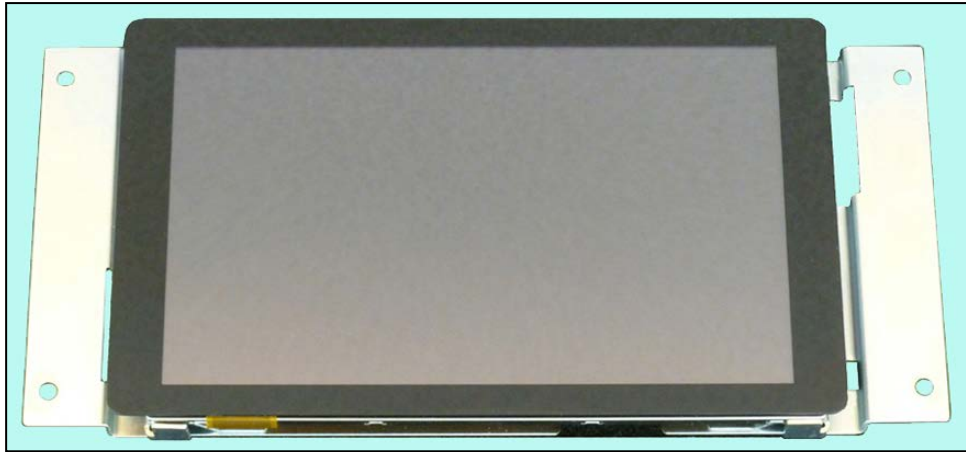
Figure 9-49. Front of touchscreen with Bracket
