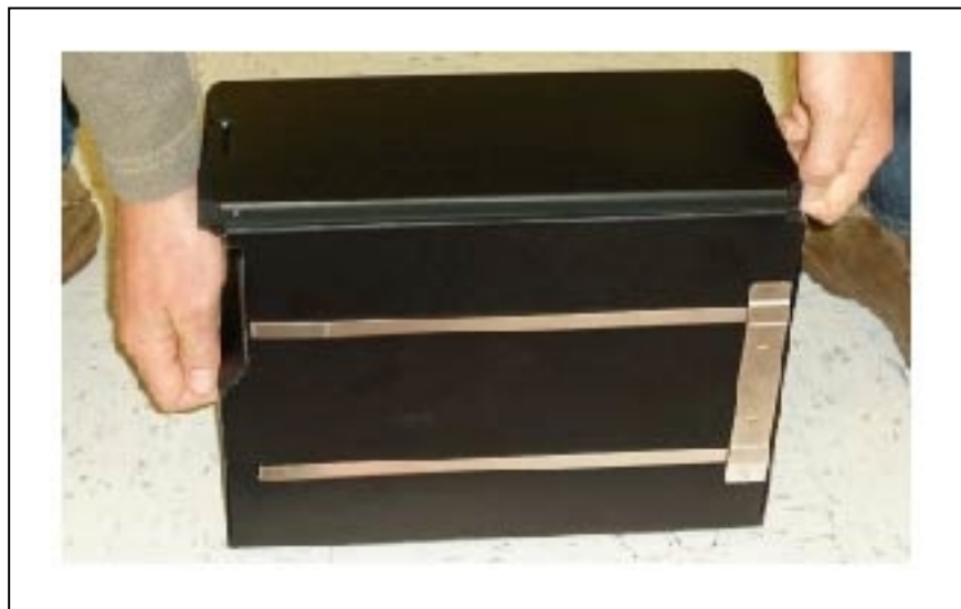
Figure 8-5. Lifting the Battery
