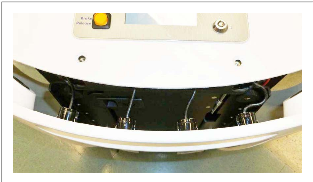
Figure 8-20. Sonar Leads, with Connectors Still in Chassis
