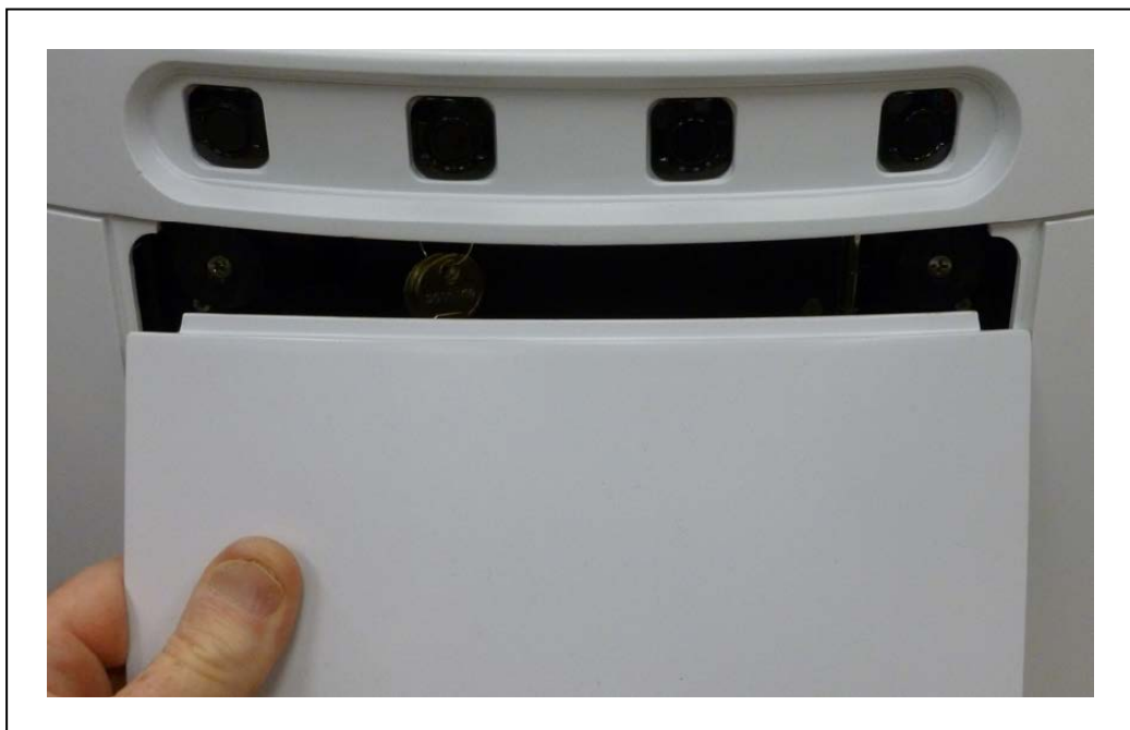
Figure 3-14. Lowering the Battery Door Platform Skin
