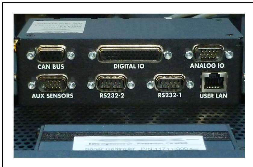
Figure 9-10. Upper Front of Core, Showing RS232 Ports
