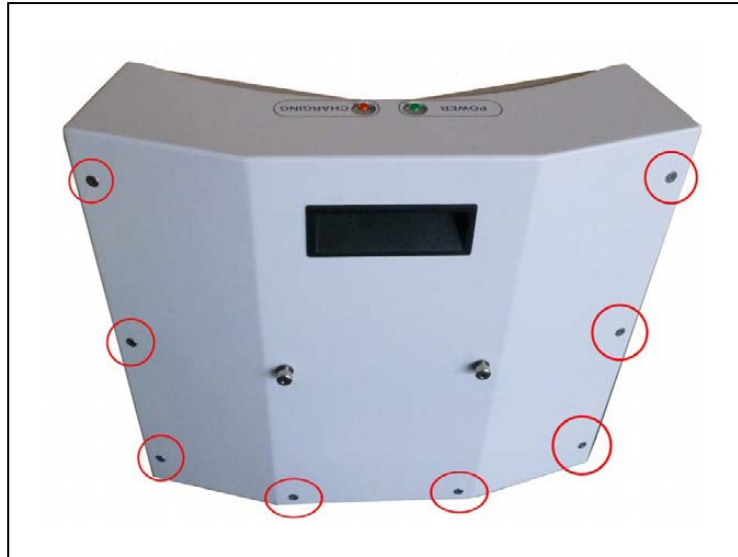
Figure 8-9. Docking Station Rear Cover Screws (8 of 10)
