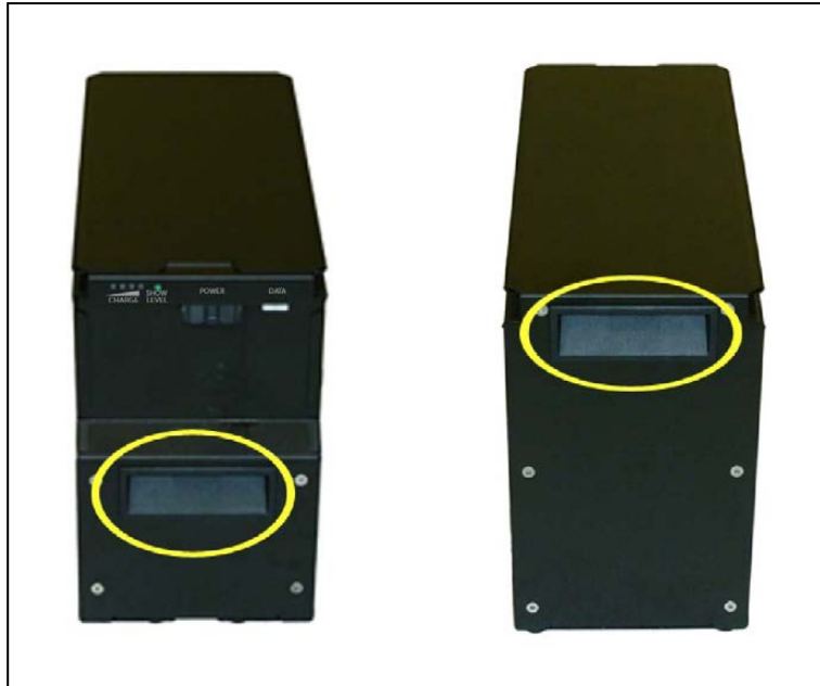
Figure 8-4. Battery Recesses, for Gripping
