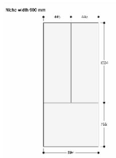
The door panel thickness is 19 mm
