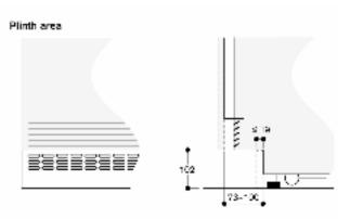
Based on the standard installation height, the height of the pinth is 100 mm.
