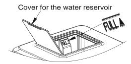
Warning: Do not pour the water into the internal water tank located underneath the ice basket. This tank is not big enough and will effect the ice making performance.
