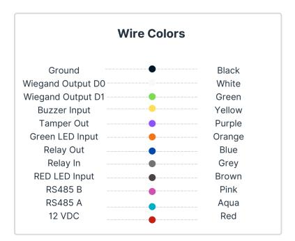
The next step is to connect the wires as per the wiring table above.
