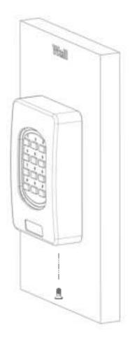
Complete the hardware installation by fixing the snake eye screws (security screws) to the top and bottom casing (#6-32X5/16" SS).
