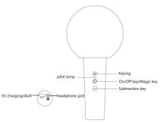
On/Off key: Press and hold for 3 seconds to turn on/off
