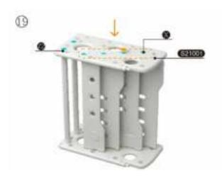
Cover the storage side panels and secure them with X small cross nut and Z2 large cross nut respectively.
