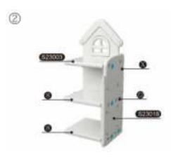
Put S23004 cabinet back board,S23003 cabinet layer and No.8 short layer board cross nut Fix and tighten S23018 to rage side plate with X small cross nut and Z2 large
