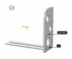
First, fix 2 storage pole to the storage side panel, Use a Z2 cross nut to secure it.
