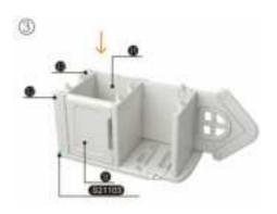
Put on the fillet buckle, put on the NO.9cabinet door panel, and plug in the cabinet backing plate And a NO.12 short leg trip
