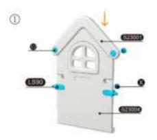
S23001 Tighten the cabinet eaveby pressing the round screw and X small cross from the top down then install the 90°screw and tighten it with X small cross,and put it aside temporarily Note the direction of the 90"screws.
