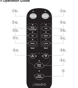
a. The "Power" button: Press this button to turn on the product with the indicator light on; Press this button again, then the product would reset (indicator light: flickering) and then shut off (indicator light: off). b. The "Heating" button: Press this button to activate the heatina function (indicator light: on) and press again to turn off the function (indicator light: off).
